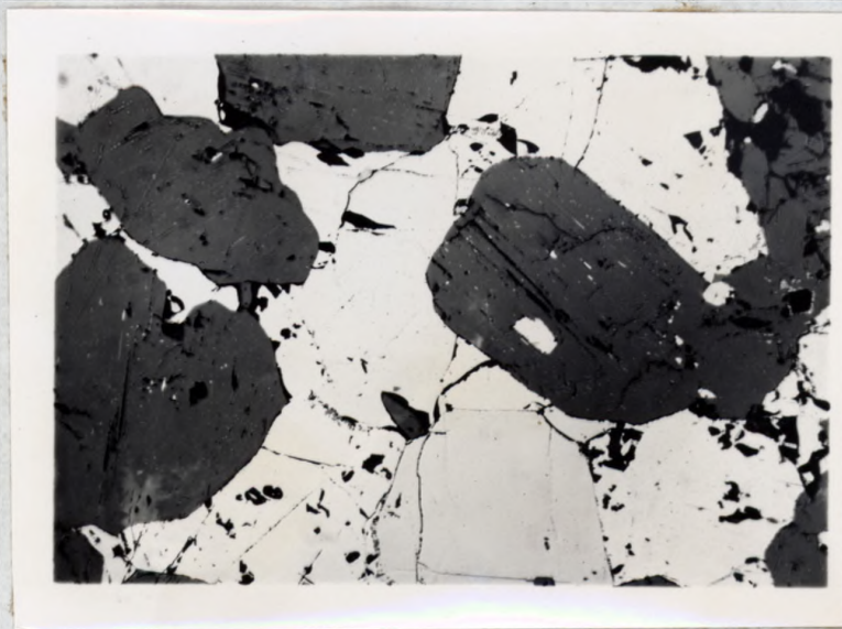
Magnetite-Ilmenite bearing pyroxenite. 28 x. Magnetite and ilmenite size: 14-65 mesh Specimen No. C-324 Polished Section No. 1141. Photomicrograph No. 347
