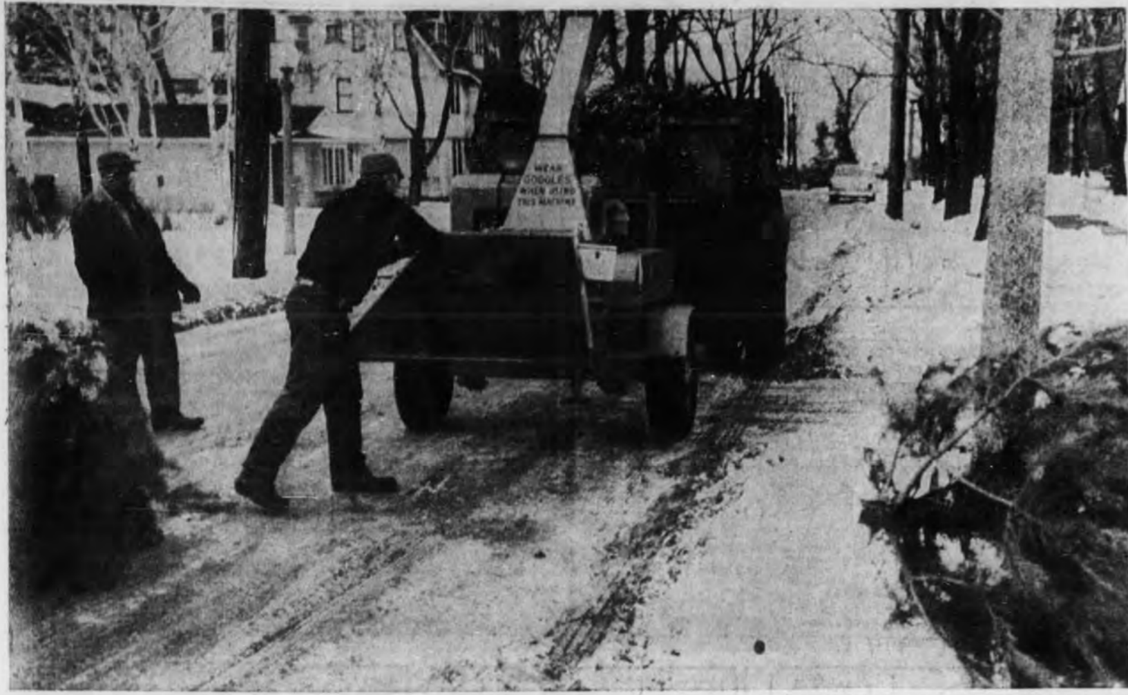
Showing a Christmas tree through the "chipper" is Paul Johnson, while another public works department employee, Clyde McVannel, watches. This picture was taken yesterday afternoon while the crew picked up trees on E. Michigan St. Trees are fed, bottom first, into
