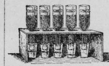
Apparatus to Test Capacity of Soils to Take in Rainfall.
