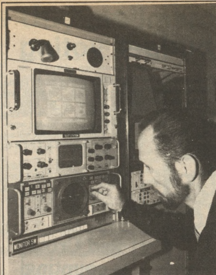
Chief Engineer Earl Littich checks the left and right channel phase relationships on the audio-visual quality monitor at WNMU TV-13. (Bernie O'Brien photo)
