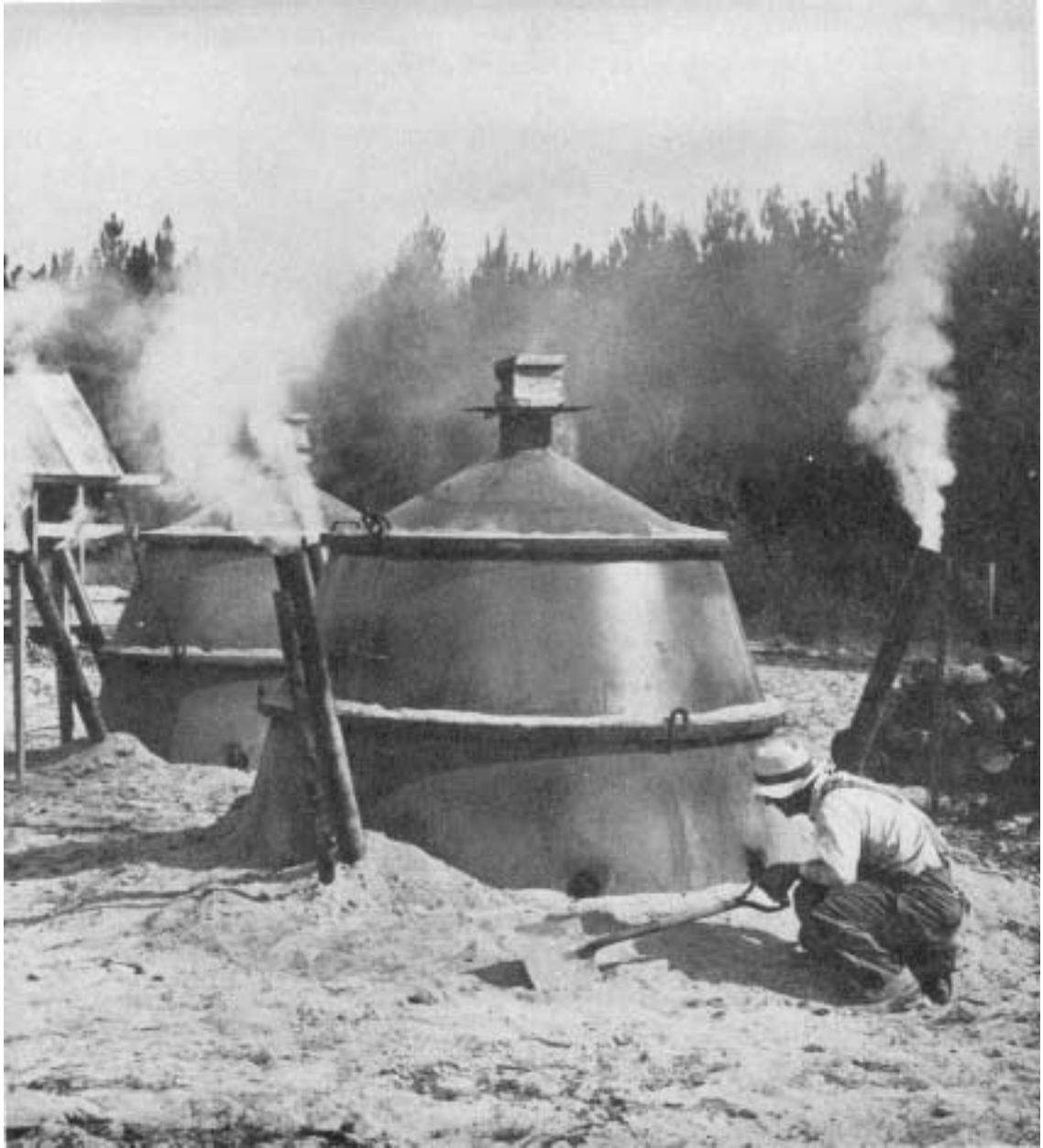
Figure 4. --Portable, sectional sheet-metal kiln.
