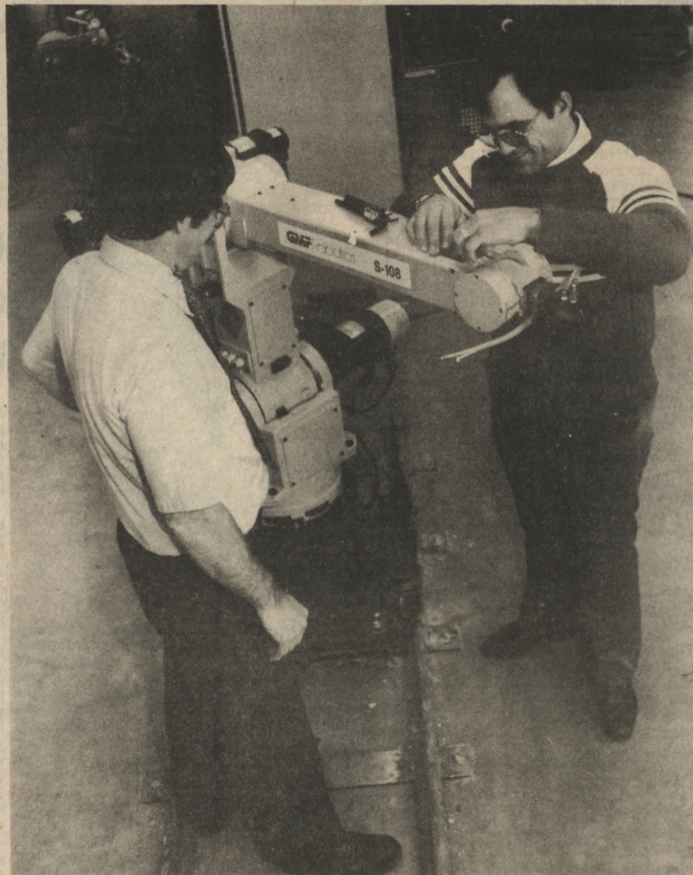
Hal Losey (right), of GMF Robotics, Inc. puts touches on installation of a new S-108 industrial robot in the Department of Industry & Technology as Prof. Thomas Meravi, robotics coordinator, looks on. One of three major types of robots used in manufacturing today, the robot represents the latest in technology and cost $40,000. (NMU photo)
