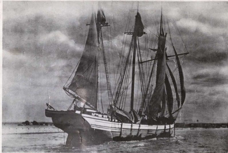
Schooner "QUICKSTEP" Entering Ontonagon Harbor 1912. Built in Green Bay, Wisconsin 1874. Length, 140 ft. 8 in.; Beam, 25 ft. 3 in.; Gross Tonnage, 282; Net Tonnage, 268. Crew of 6 men.
