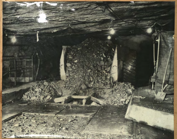
DUMPING THE ORE ONTO CONVEYOR BELT AT A DUMP STATION
