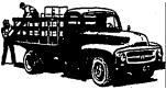
STAKE, R-110 Series, Heavy Truck bed floor, 216 inch wheel base. 16 1/2" wheel base. Sturdy steel stake easily removable for flat-bed operation.
