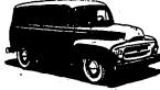
PANEL, R-110 Series, 115-inch wheelbase. Load-carrying capacity: Length 90 inches, width 20 inches, height 54 inches. Rear doors open to 90° or 180 degree position.
