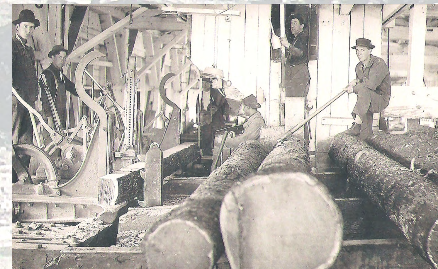
Logs were cut into lumber and sent to big cities, like Chicago. Slab wood (bark edges) was sold to residents for $1.25 a cart load for stove wood.
