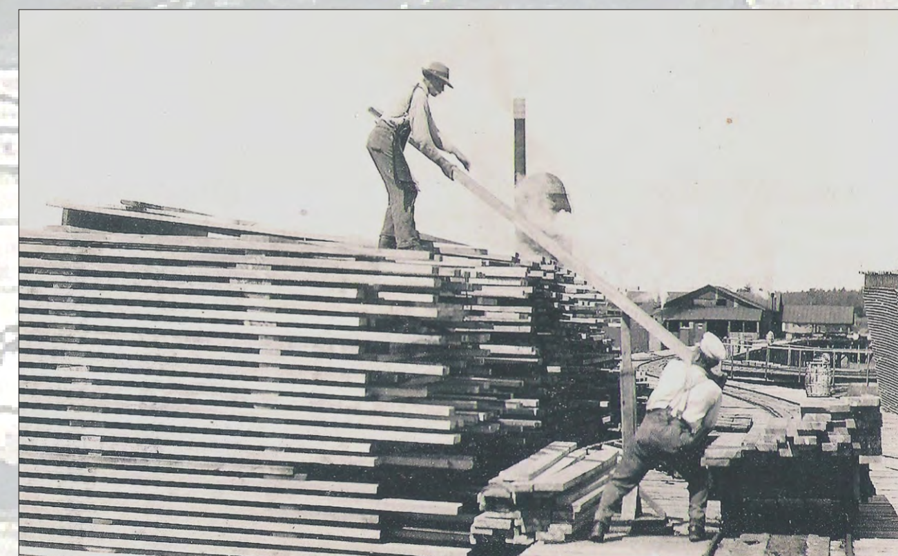
Lumber was stacked by hand on the docks to await loading on ships.
