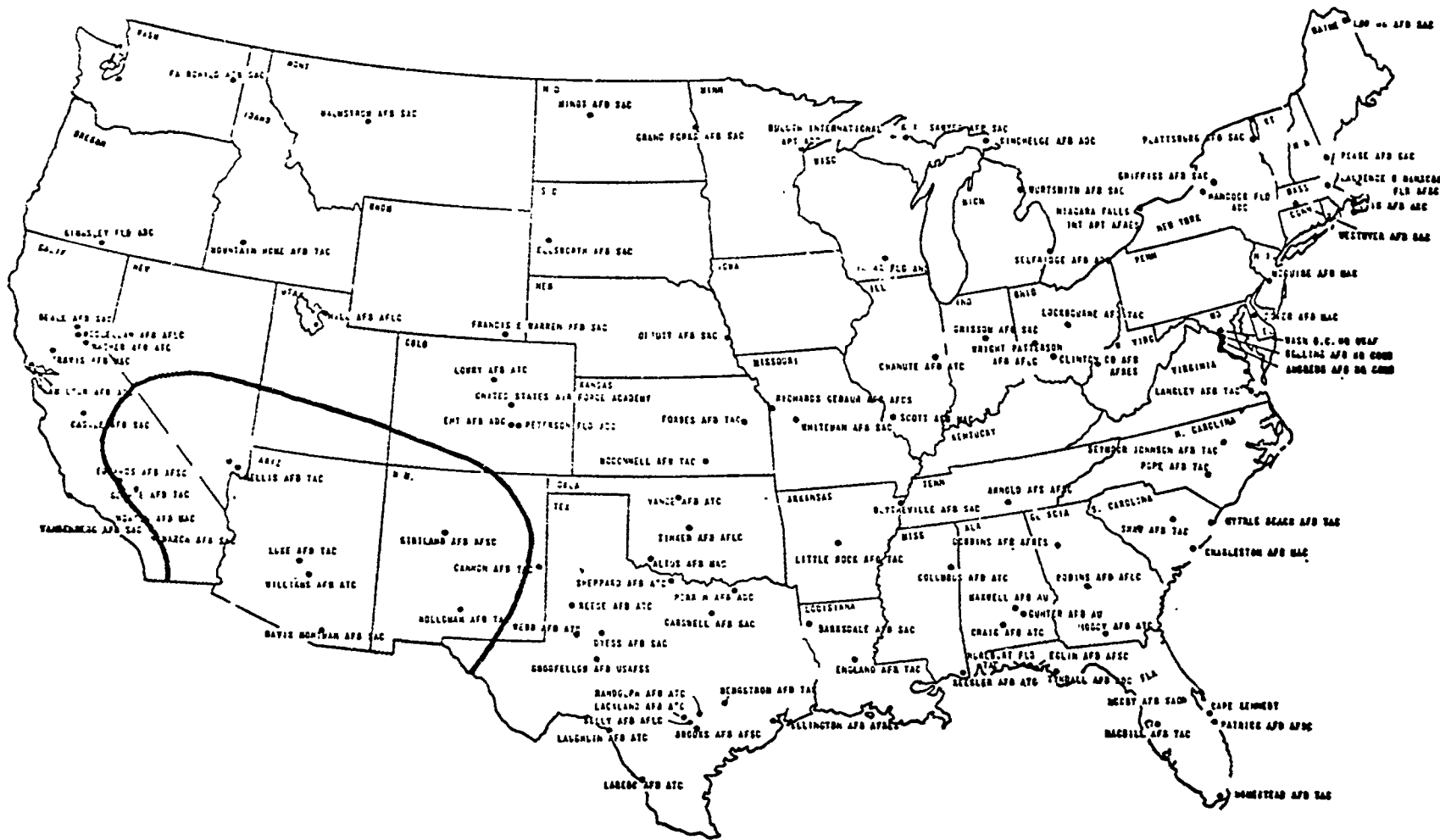
Figure 10. Potential Solar Thermal Electrical Conversion System Region. This figure is merely intended to show the general geographical area which possesses good potential for solar thermal systems. Other locations may exhibit potential upon further analysis of the direct normal radiation component when tilting and/or tracking is taken into consideration.
