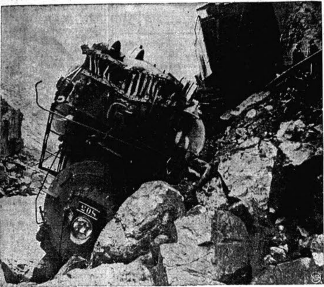
When a lot of locomotive meets a lot of rock, it's just too bad for the locomotive. Here's what happened when a Denver and Rio Grande Western passenger train smashed into a 40-ton boulder that had roared down the side of the famed Royal Gorge in Colorado and stopped on the railroad tracks. The locomotive is shown dumped upside down into the Arkansas river. The rest of the train stayed on the track and all passengers were unhurt, but the engineer was killed and the fireman badly burned.
