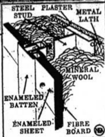
Above is a sketch showing the porcelain-enamel house being erected in Cleveland, Ohio. Lower right is a diagram showing how the enameled sheet-metal plates are assembled.
