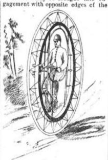
IMLAR'S UNICYCLE. double rim. the roller coming in contact with one edge of the rim. turning the wheel in the opposite direction. and when engaging the other edge moving the wheel in the reverse direction. One can easily get into the machine by turning the framework half way around, allowing the saddle to come back into place after stepping in. -Scienlific American.
