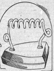
vantages over any other form, of fixed handle iron. It is stated that the coil forming the handle is so arranged that in making the circles just above the body of the iron the metal surfaces do not touch, and as a result the heat is thrown off and does not enter the handle as it otherwise would.
