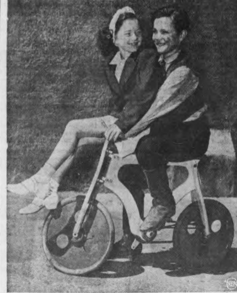
Two Los Angeles youngsters demonstrate a bicycle built of wood to meet the shortage of bikes. Three metal bolts hold the vehicle together and it runs on tires of reclaimed rubber.
