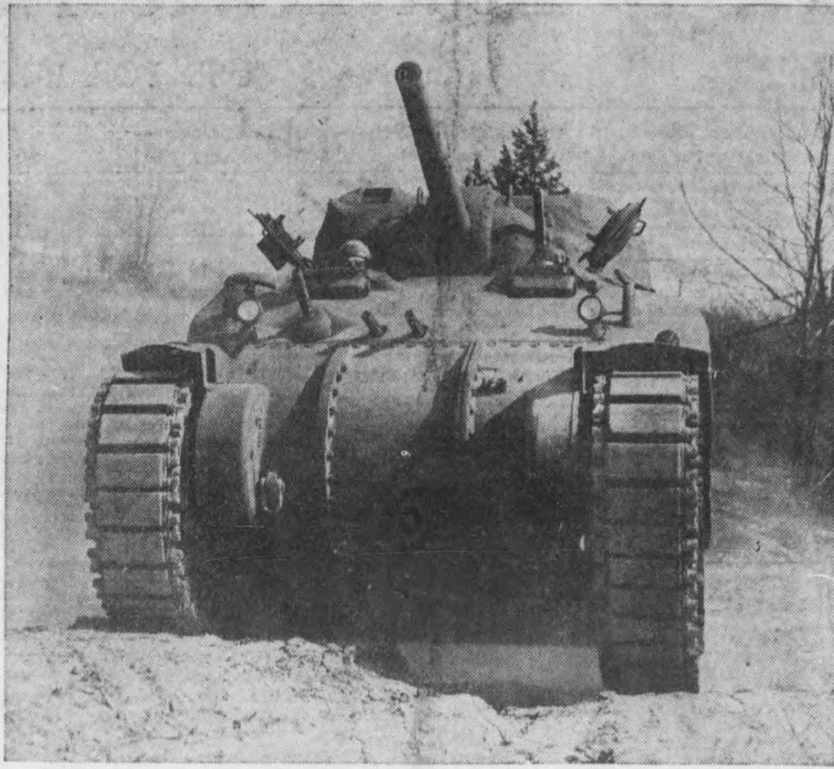
Thundering over a ridge at Fort Knox, Ky., testing ground comes the Army's new rivetless medium tank complete with 75 mm. gun and a battery of machine guns. The M-4 has an all-cast body and mounts its big gun on revolving turret in center instead of lower down on the right side as on the M-3 tank.
