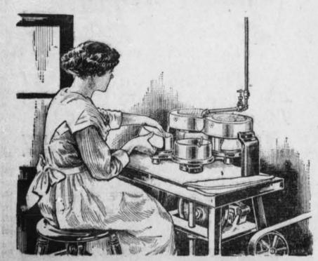
We are first to install the above machine for finishing the popular Turn down collar. Before producing the collar sufficient moisture is given which in sures its being turned and moulded into shape without cracking. The outer collar is separated from the band so that a space is moulded between, making ample space for the tie to slip freely-SOME COMFORT. We believe this method of producing collars will eliminate the cracking and add to the life
