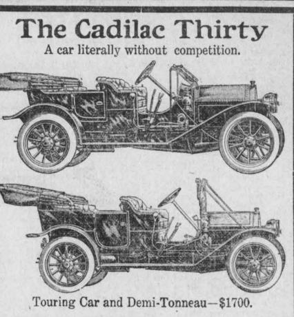
Wheel base, 116 inches. Bore, 41/2x41/2. Horsepower, A. L. A. M. Rating, 32.4. Double Ignition System. Bosch Magneto. Wheels, 34x4. Timken Roller Ball Bearing. Speedometer. Full set of Tools
