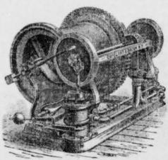
"BACON'S" REVERSIBLE AND FRICTION WINDING ENGINES FOR MINES. "MINING PLANTS." CONCENTRATING WORKS.
