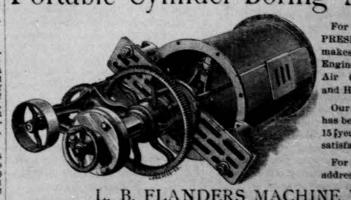
For boring IN THEIR PRESENT POSITIONS all akes and sizes of Steam Engine Cylinders, Pumps, Air Compressors, Mining and Hoisting Engines, etc.
