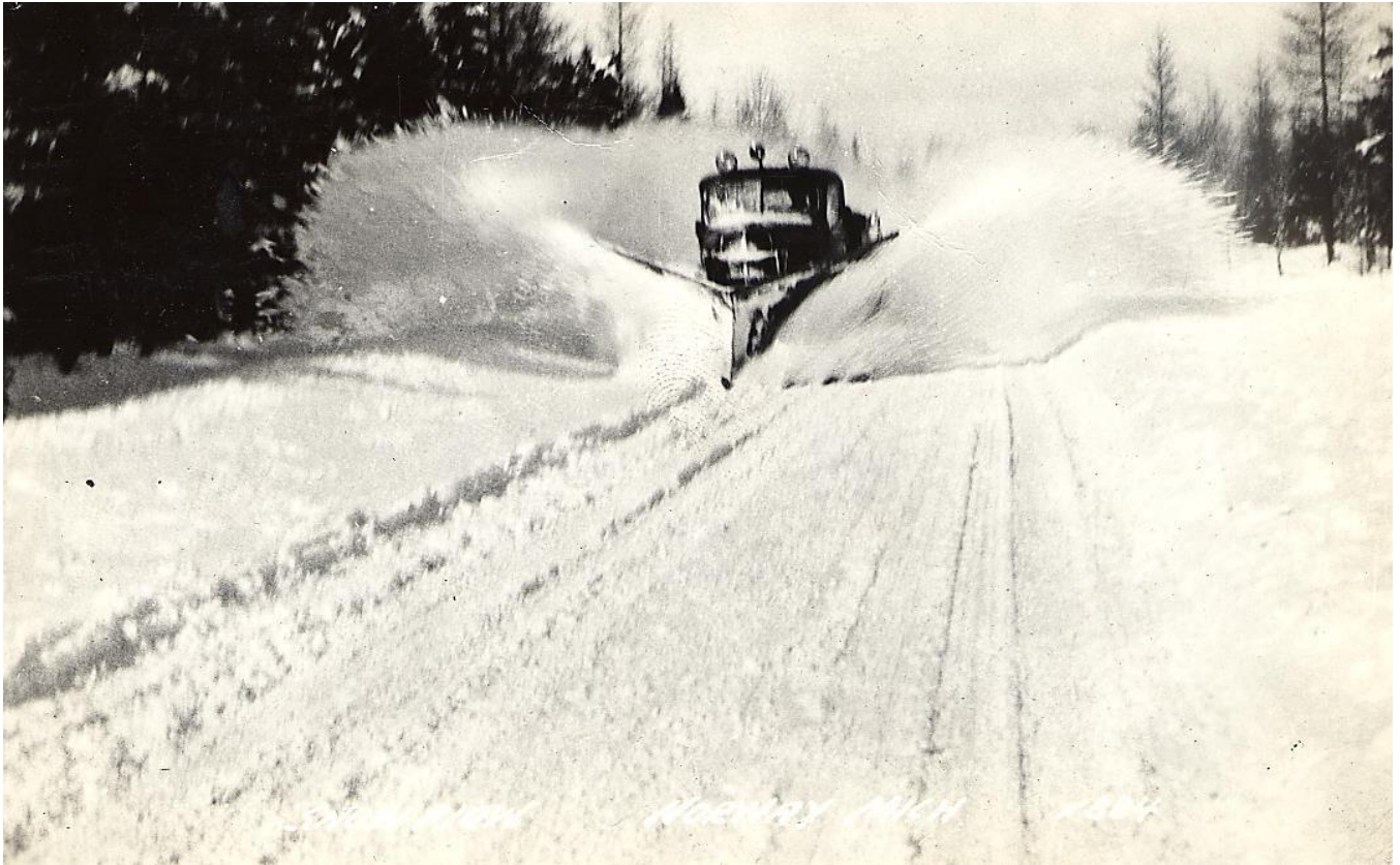
Snowplowing with V-Shaped Plow, Norway, ca. 1945: Postmarked Norway, Mich., November 19, 1945, this postcard view shows a V-shaped plow clearing the highway following a snowstorm with snow flying in both directions. [William John Cummings]
