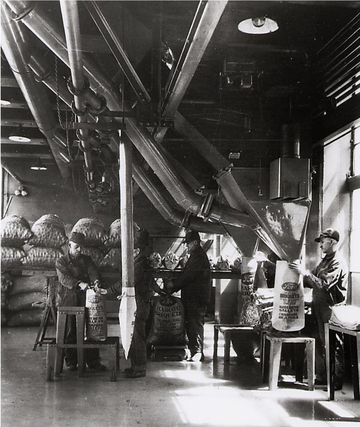
Ford Motor Company, Chemical Building, Bagging Ford Charcoal Briquettes, Kingsford, ca. xxxx: Workers are filling bags with charcoal briquettes, one of the by-products of the Ford Motor Company's manufacturing plant in Kingsford. After Ford left, the manufacture of briquettes continued under the brand name Kingsford Charcoal Briquettes. [Jack Deo, Superior View Studio]
