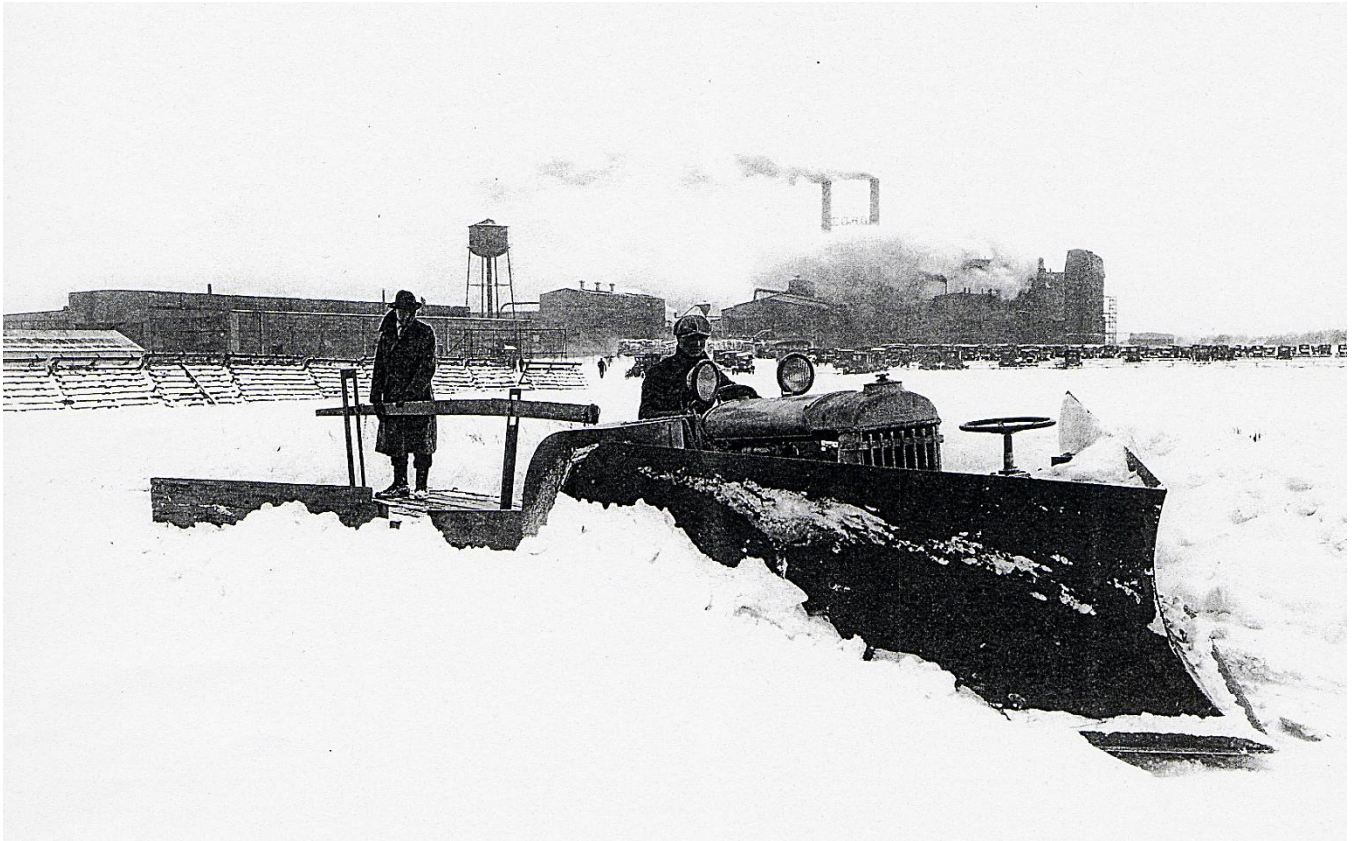
Ford Motor Company Plant in Kingsford, Looking Southwest, ca. 1925-1930: A Fordson tractor was pushing the snowplow on the northeastern side of the Ford Motor Company's plant in Kingsford. Note the cars in the parking lot behind the tractor. [William John Cummings or Guy Forstrom]
