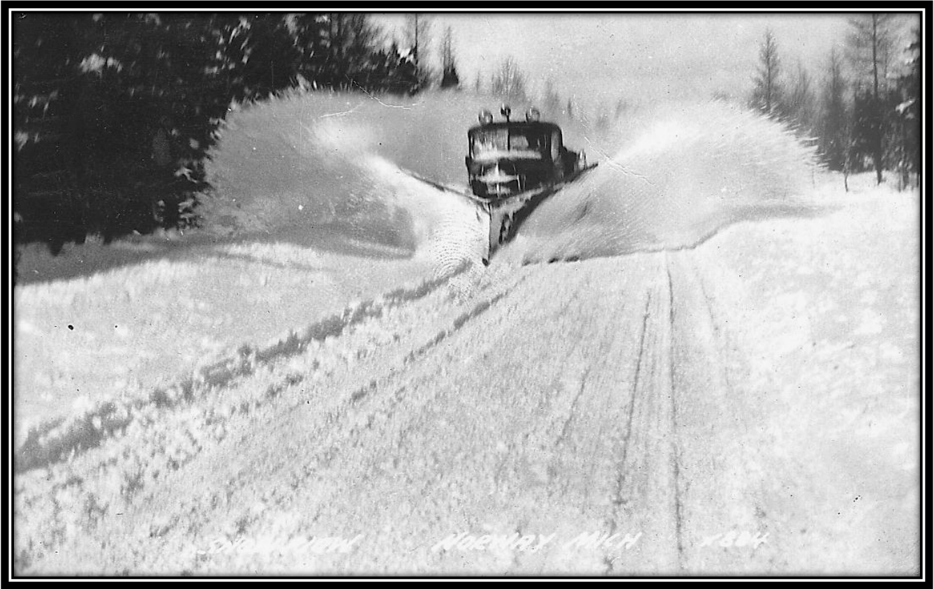
Postmarked Norway, Mich., November 19, 1945, this postcard view shows a V-shaped plow clearing the highway following a snowstorm with snow flying in both directions. [WJC Photo]
