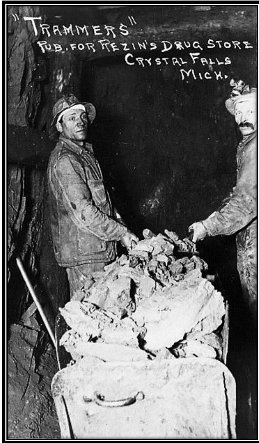
“Trammers” Crystal Falls, Iron County, Michigan, ca. 1922: This real photo postcard view identified as “Trammers’ Pub. For Rezin’s Drug Store, Crsytal Falls, Mich.” is postmarked Crystal Falls, Michigan, April 4, 1922 and shows a rare interior mine view with two trammers whose job was to fill the small underground ore cars to the shaft to be hauled to the surface. The miner at the right has a carbine lamp on his hat. Note the headbands worn under the hats. [William J. Cummings]
