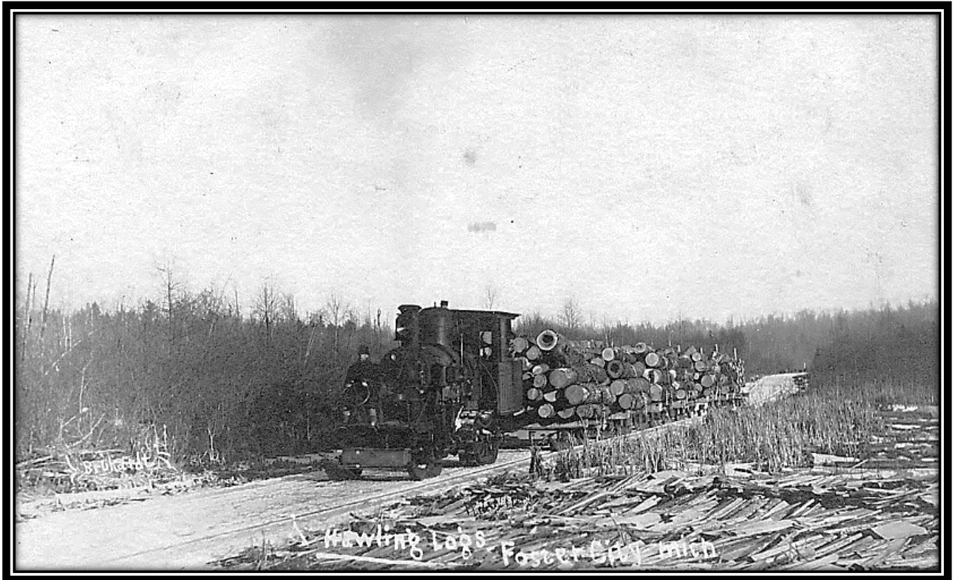
Morgan Lumber & Cedar Company Steam Hauler, Near Foster City, Dickinson County, Michigan, ca. 1910-1915: This unused real photo postcard view identified as “ Hauling Logs, Foster City, Mich. ” shows the Morgan Lumber & Cedar Company’s steam hauler near Foster city and dates from between 1910 and 1915. Traveling on man-made ice roads which were sometimes sanded if conditions warranted it, a steam hauler hauled 15 to 20 loads at a time on day and night shifts, bringing logs and “short stuff” from the camps to the company’s mill in Foster City. This photograph was taken by Brulardt (Ernest Robert Brukaradt, amateur photographer who worked as a railroad station agent in Felch) name appears just above the road at the lower left corner. [William J. Cummings]
