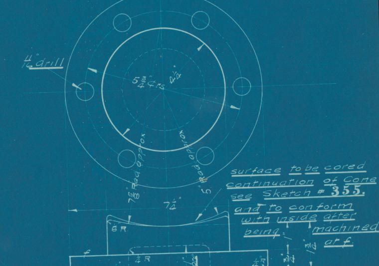
23 core \_ Allow for finish on surfaces marked fonly
