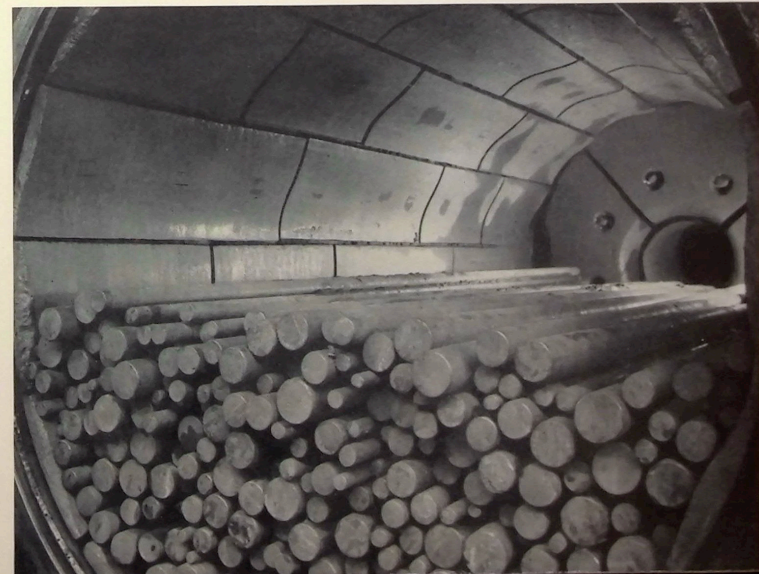
Rod Mill with head removed to show rods.
