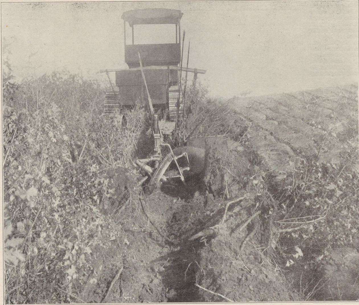
A Powerful International Tractor Pulling a P. & O. Grub Breaker That is Turning Everything Under
